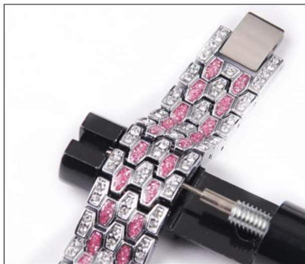
02: Remove extra links- Align the pin inside the band to tool needle according the arrow direction showing in picture, rotate the tool wheel to push the pin out.
