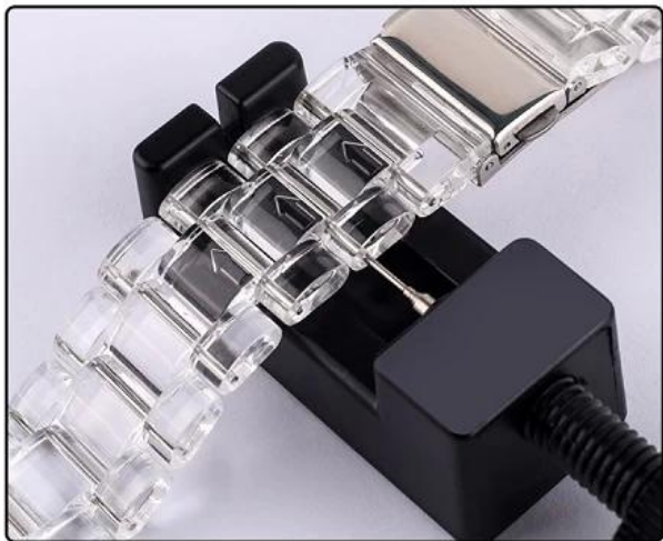
Remove bracelet links as the arrow indicate
