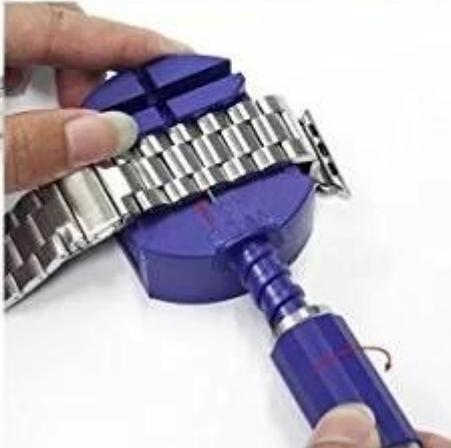
1. Place the tip of the hole, punch into the hole of the link, twist right to press the link bar out through the opposite side;
