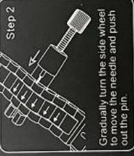
Gradually turn the side wheel to move the needle and push out the pin.
