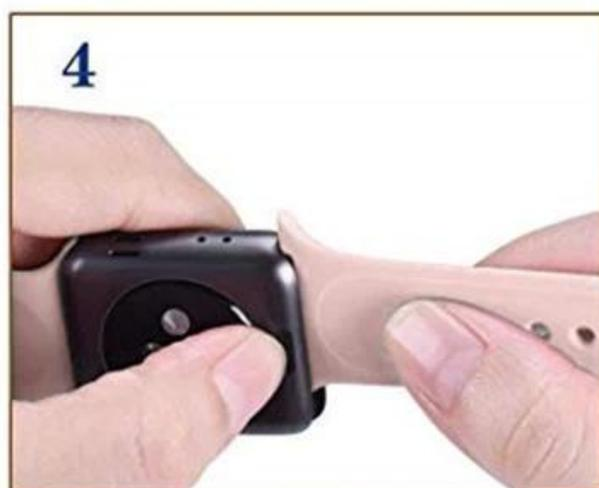
Press the release button to slide out
