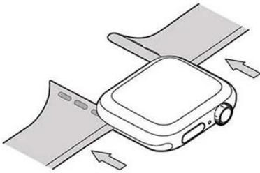
1. Remove the straps from the base of the watch.
