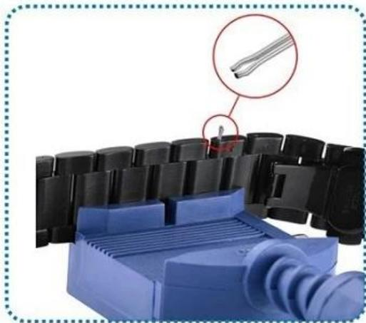
3. Reinstall the pin into the band, the direction of arrow is contrary to the Step 1
