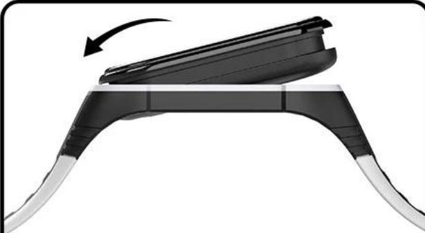
1. Put one side of host along the dent into strap.
