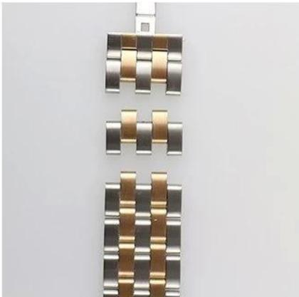
5. Assemble links. Put 1 of the rod end to the hole inside another link, then align the 2 links.
