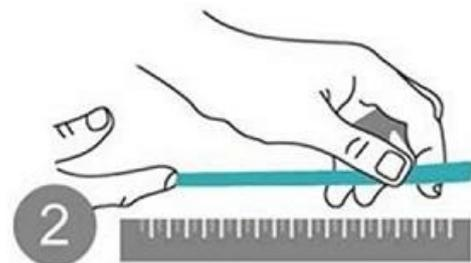
Measure the rope length from zero scale to the marked position with a ruler.
