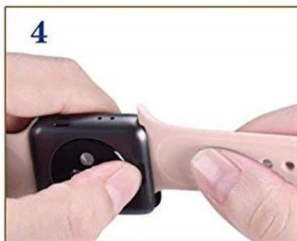
Press the release button to slide out
