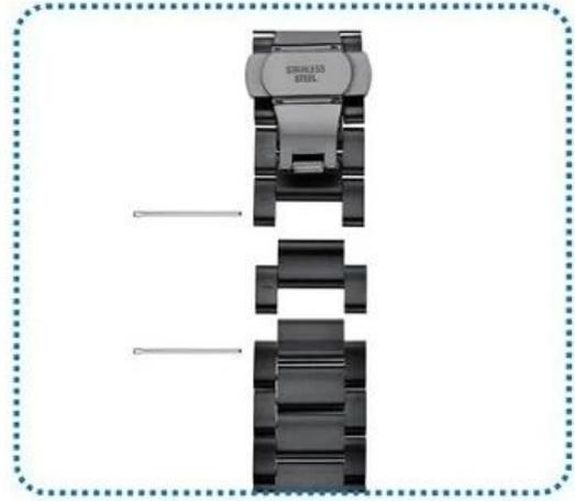
2. Pull out the pin from the other side and remove links
