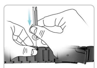
4.Use the tool to press down the spring bar and push the link in. Then loosen the tool and slightly adjust the link to make both sides of the spring bar buckle firmly. Finally, the installation is successful.
