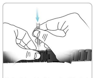
1.Use the tool to insert the band hole, press down slightly and push out the link ,with link is removed successfully.
