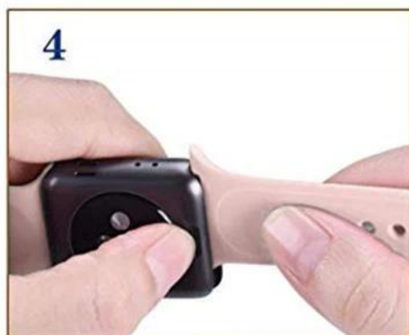
Press the release button to slide out
