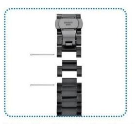
2.Pull out the pin from the other side and remove links
