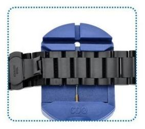
4. Put the links in the pin link remover and use it to push the last side of the pin
