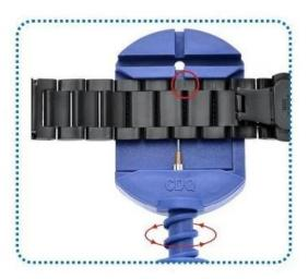
Make the side with printed arrows face up, use the tool to push out the pin
