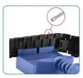
3. Reinstall the pin into the band, the direction of arrow is contrary to the Step 1
