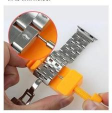
3. Twist clockwise the link remover to press the link bar out with the direction of arrow. And then pull out the link bar out of it with your hands.
