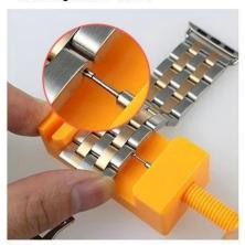
6. Use the link remover to push the elastic rod in so the link will go into another. Slightly adjust the link position until they locked firmly.
