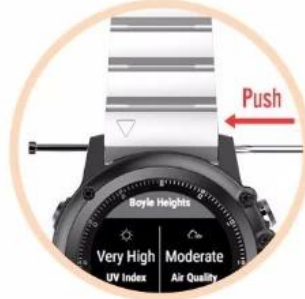
2. Push the spring bar out.
